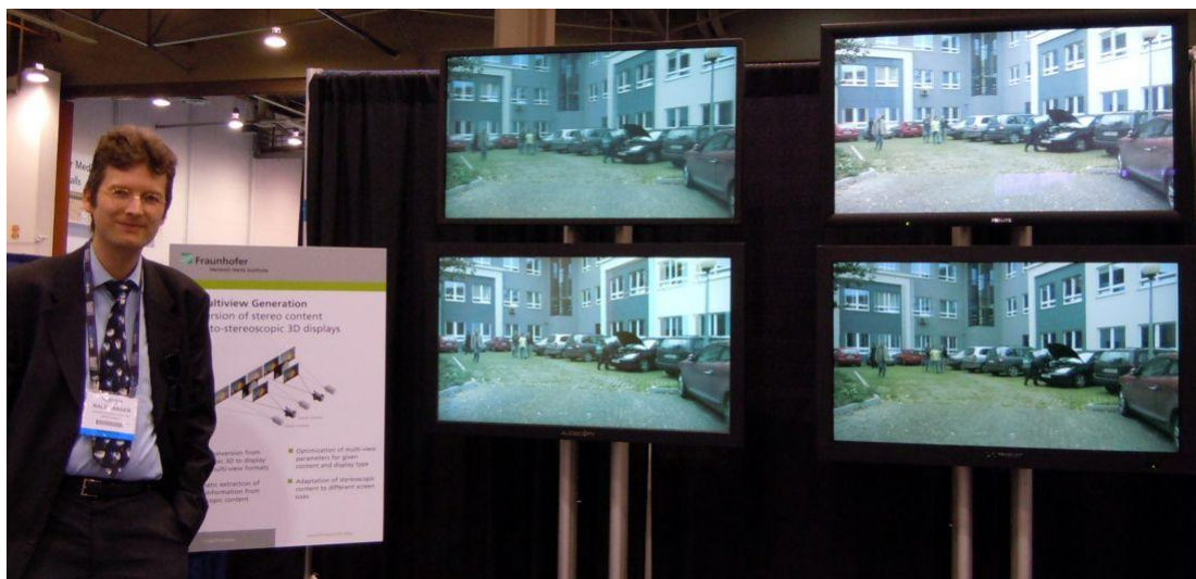
Ralf Tanger of the HHI (Heinrich Hertz Institute) branch http://www.hhi.fraunhofer.de of the world famous German R&D institute Fraunhofer (both with long histories of 3D projects) showing their new autostereoscopic server software playing from one file on 42 inch panels from four different auto panel makers--Tridality www.tridality.de (5 view barrier), Alioscopy www.alioscopyusa.com (8 view lenticular), NewSight www.newsight.com (8 view barrier) and Philips (terminated this product line a year ago) (9 view lenticular). Fraunhofer has been researching 3D for at least a decade and the HHI long before that. They also showed multiview synthesis from two views (e.g., from a stereo
