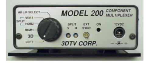
The Model 200 selects one of two sets of inputs and applies it to the outputs in a field alternate manner, i.e., the left field is output from INS-1 and the right field is output from INS-2.
