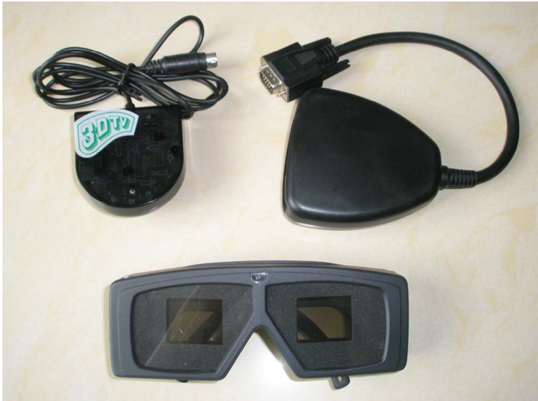
Fig 6. The TriD dongle is usable with any kind of wired or wireless LCD shutter glasses. For wireless glasses the Quad Mode transmitter shown here is required.
