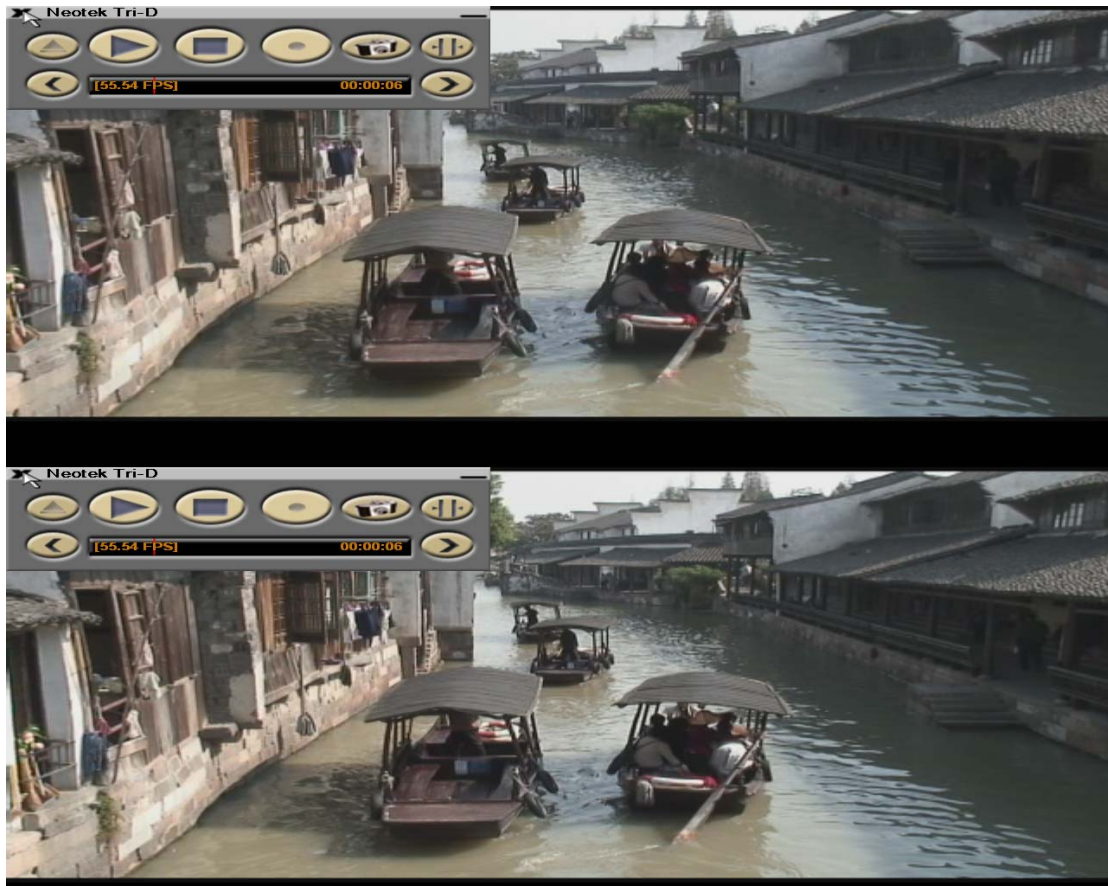
Figure 1. The above/below image format used by TriD as it will appear on a non 3D display like LCD monitors or on CRT's when the dongle is not used or sync pulse is not being inserted. Shown in the toolbar are the forward and reverse arrows, the black timeline bar with red time position line, FPS capture rate and time.
