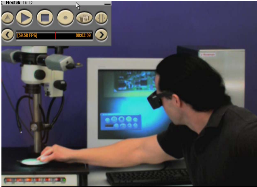
Figure 2. Screen capture of live 3D video in the overlapped frame sequential format with the GUI(toolbar) in upper left (which appears by clicking anywhere on the screen). Shown with the Bunton Group 3D video microscope system. The 60hz/eye 120hz frame sequential images, with properly aligned cameras, overlap perfectly as shown so that the image appears almost like a single 2D image. For field use with a laptop or with LCD or Plasma displays, the right and left images will also overlap when viewed in alpha blend mode.
