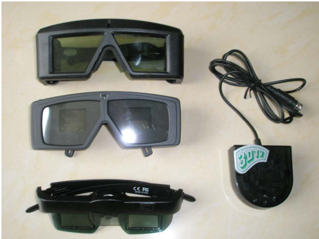
Fig. 7 The Universal Wireless Transmitter with 3 kind of glasses.
